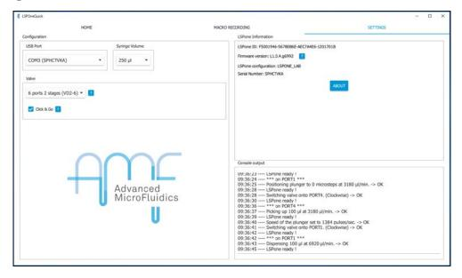
The settings tab allows you to input which specific pump configuration you are using:
