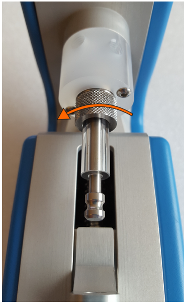
FIGURE 4.3 – Insertion of the syringe removal tool around the glass barrel. Unscrew the syringe by turning in the highlighted direction.
