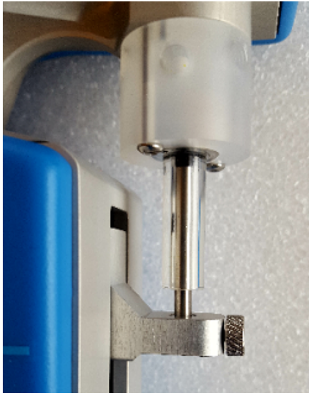
FIGURE 4.6 – Correct plunger lock screw fixation
