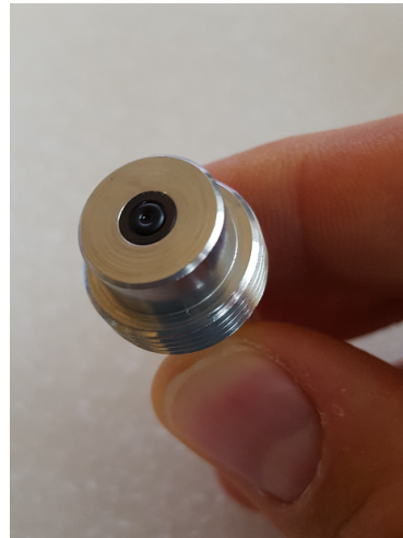
FIGURE 4.4 – Syringe seal to be handled with care. Before screwing the syringe, ensure that the black O-ring is correctly inserted in the groove as shown here
