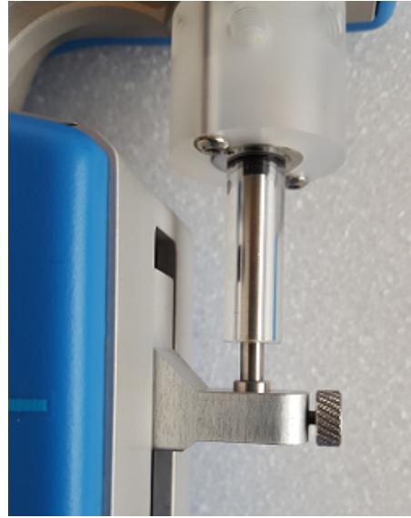
FIGURE 4.7 – Incorrect plunger lock screw fixation
