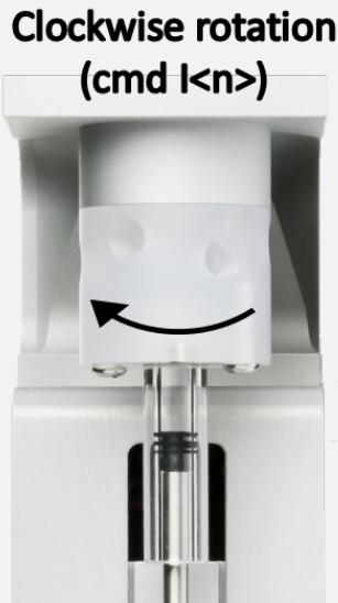
FIGURE 3.7 – Direction of rotation definition for the plug - clockwise rotation corresponds to a 60° rotation when incrementing the port number by 1, counterclockwise rotation corresponds to a 60° rotation when decrementing the port number by 1
