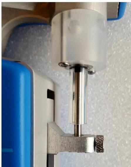
FIGURE 4.5 – Correct plunger lock screw fixation
