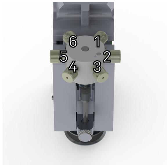
FIGURE 3.2 – Cut section revealing port numbering
