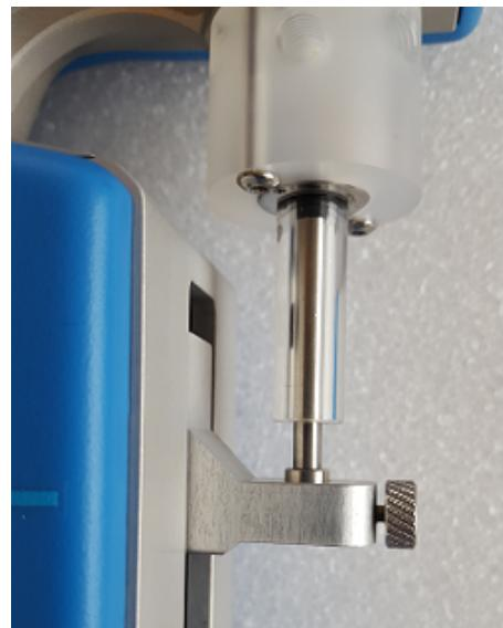
FIGURE 4.6 – Incorrect plunger lock screw fixation
