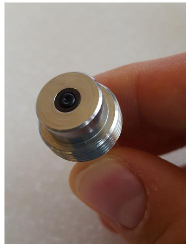
FIGURE 4.3 – Syringe seal to be handled with care. Before screwing the syringe, ensure that the black O-ring is correctly inserted in the groove as shown here
