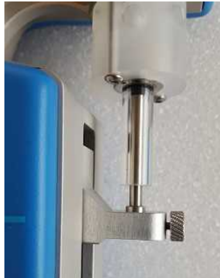
FIGURE 4.10 – Incorrect plunger lock screw fixation
