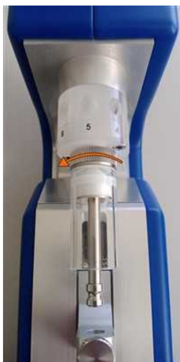
FIGURE 4.6 – Unscrew the syringe using fingers friction against the knurl
