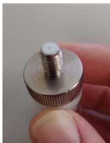
FIGURE 4.7 – Syringe seal to be handled with care. Before screwing the syringe, ensure that the PTFE surface is clean and not scratched
