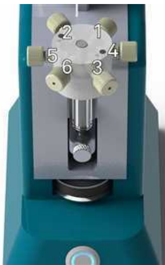
FIGURE 3.5 – Cut section revealing port numbering - VD2-6
