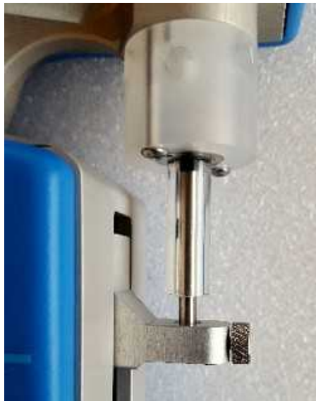
FIGURE 4.9 – Correct plunger lock screw fixation
