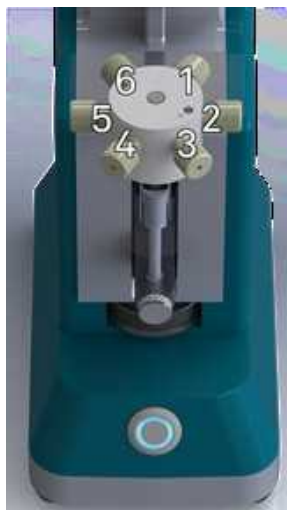
FIGURE 3.2 – Cut section revealing port numbering - VD1-6
