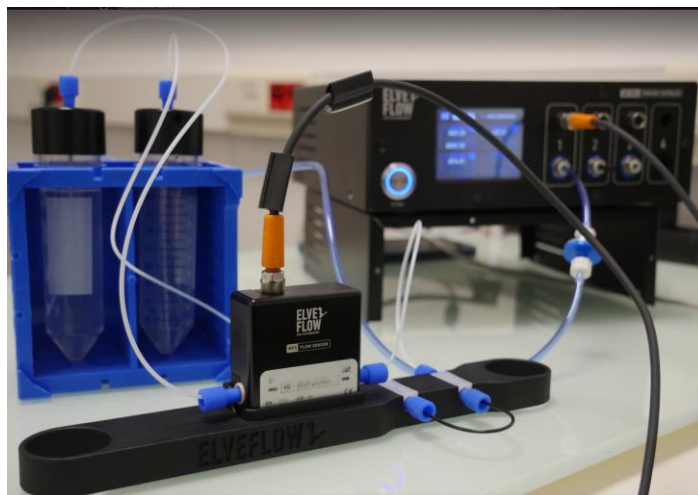
Figure 1 – Illustration of the experimental set-up used to calibrate an MFSD4 using an OB1 MK4 pressure controller (0-2bar channels), 100µm fluidic resistance and 1/16" OD PTFE tubing
