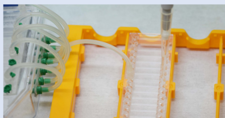
Before starting your experiment, flush the chambers with ethanol and media to remove air from the wells.
