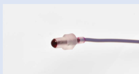
Before assembling the tubing to the chip, make sure all air has been removed from syringes and tubing by forming a droplet at the end of the connector.
