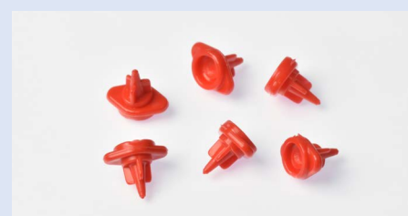
When sealing unused inlet interfaces, apply Mini Luer plugs with low volume displacement. Fill the inlet interface with media before applying the plug to avoid trapping air.
