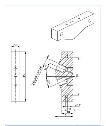
DescriptionArticle no.Manifold UNF ¼"-28 PEEK (low internal volume)695956 ≒
