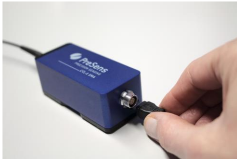
Fig. 2 Connecting the USB cable
