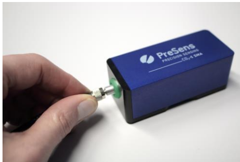
Fig. 1 Connecting the SMA plug to the CO 2 -1 SMA
