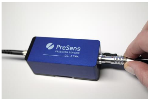
Fig. 3 Connecting the temperature sensor to CO 2 -1 SMA
