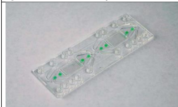
Figure 16: Cross-flow membrane chip 653 with oxygen-sensor spots
