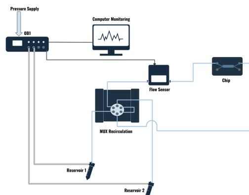
**Illustration and setup principle to perform fluid recirculation with an Elveflow MUX Recirculation valve.** The detailed protocol for this application can be found in the MUX Recirculation valve user guide.
