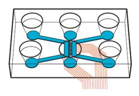
The DuaLink™ Shift MEA is a 3-compartments chip, with asymmetrical shape, connected by microchannels *tunnels* technology that allow discontinious connectivity and synaptic isolation, crowned on a MicroElectrod Array (MEA) Plate.
