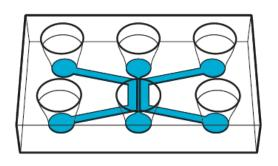
The DuaLink<sup>TM</sup> is a 3-compartments chip connected by microchannels *tunnels* technology that allow a discontinious connectivity.
