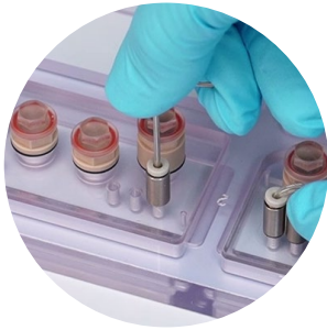
7 Screw in HUMIMIC TubeAdapters.
