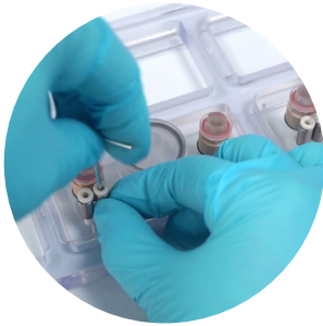
7 Screw in HUMIMIC TubeAdapters.
