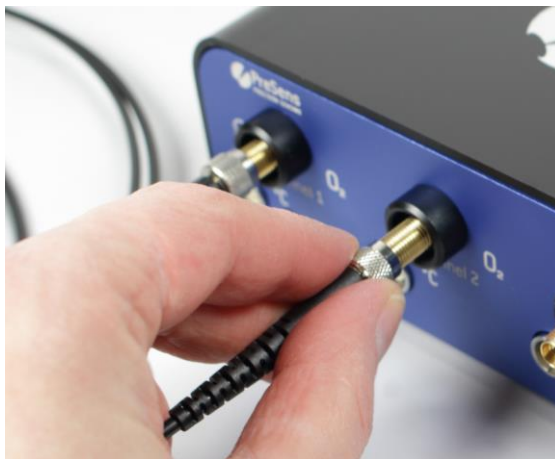
Fig. 1 Connecting the SMA plug to the connector on an MCR-O2P1C1
