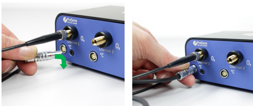
Fig. 4 Connecting the temperature sensor to an MCR-O2P1C1
