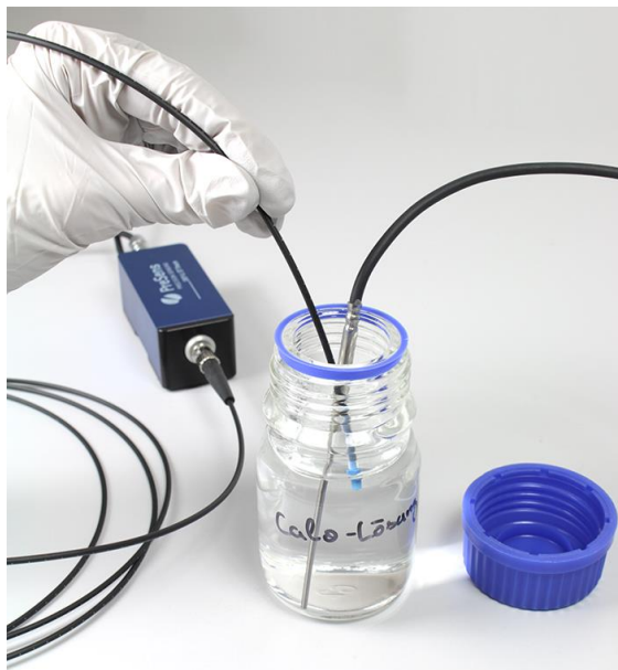
Fig. 6 Calibration set-up: The SPL is connected to the oxygen meter and held into a vessel with calibration solution.
