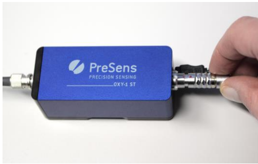
Fig. 3 Connecting the temperature sensor to OXY-1 ST
