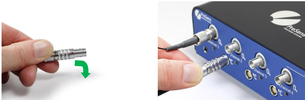
Fig. 4 Connecting the temperature sensor to OXY-4 ST
