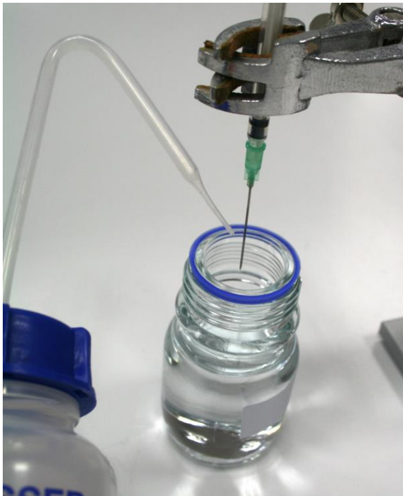
Fig. 14 Wash the NTH with distilled water if the needle had been dipped into water with sodium sulfite
