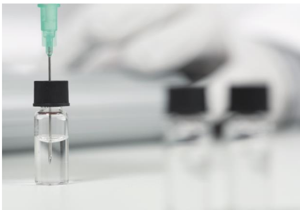
Fig. 3 Needle-type oxygen microsensor pierced through septum rubber of a pharmaceutical vial
