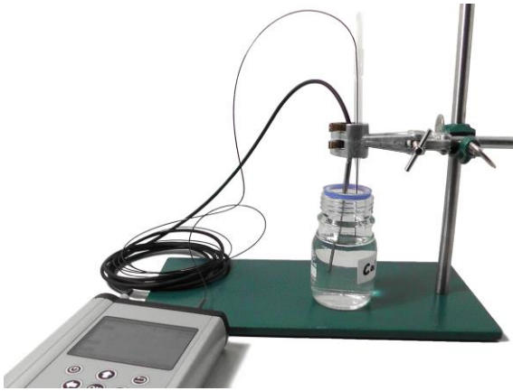
Fig. 21 IMP and temperature sensor placed in calibration standard 0 (Cal 0)
