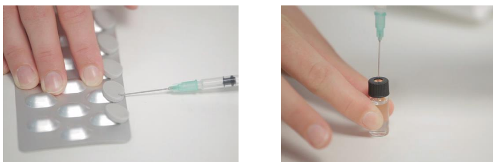
Fig. 17 Measurement with a needle-type oxygen microsensor in a blister and a pharmaceutical vial – the syringe needle is pierced through a septum, then the sensor tip is extended.
