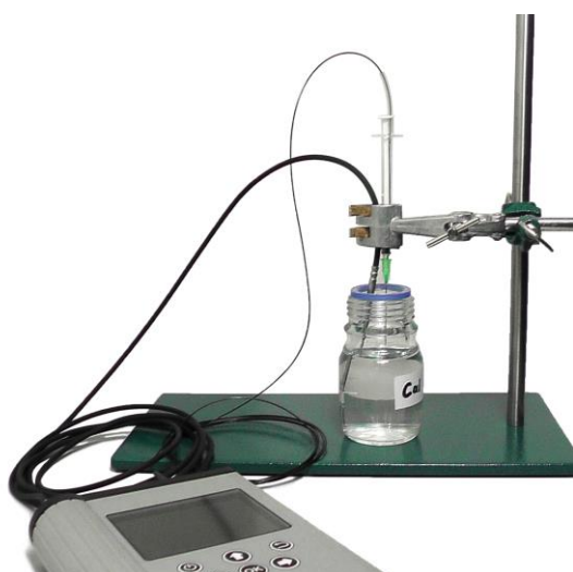
Fig. 12 NTH and temperature sensor placed in calibration standard 0 (Cal 0)
