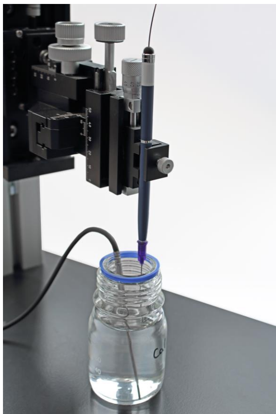
Fig. 27 PM and temperature sensor placed in calibration standard 0 (Cal 0)
