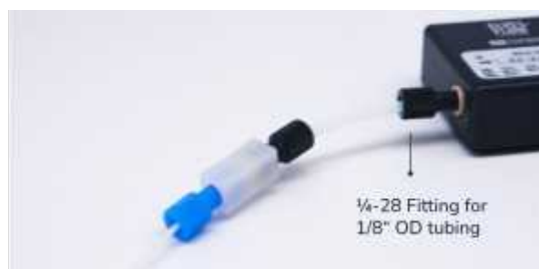
Fig 12. Recommended mounting for MFS5
