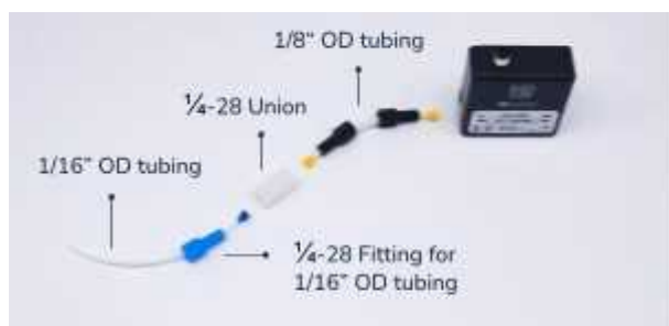
Fig 12. Recommended mounting for MFS5
