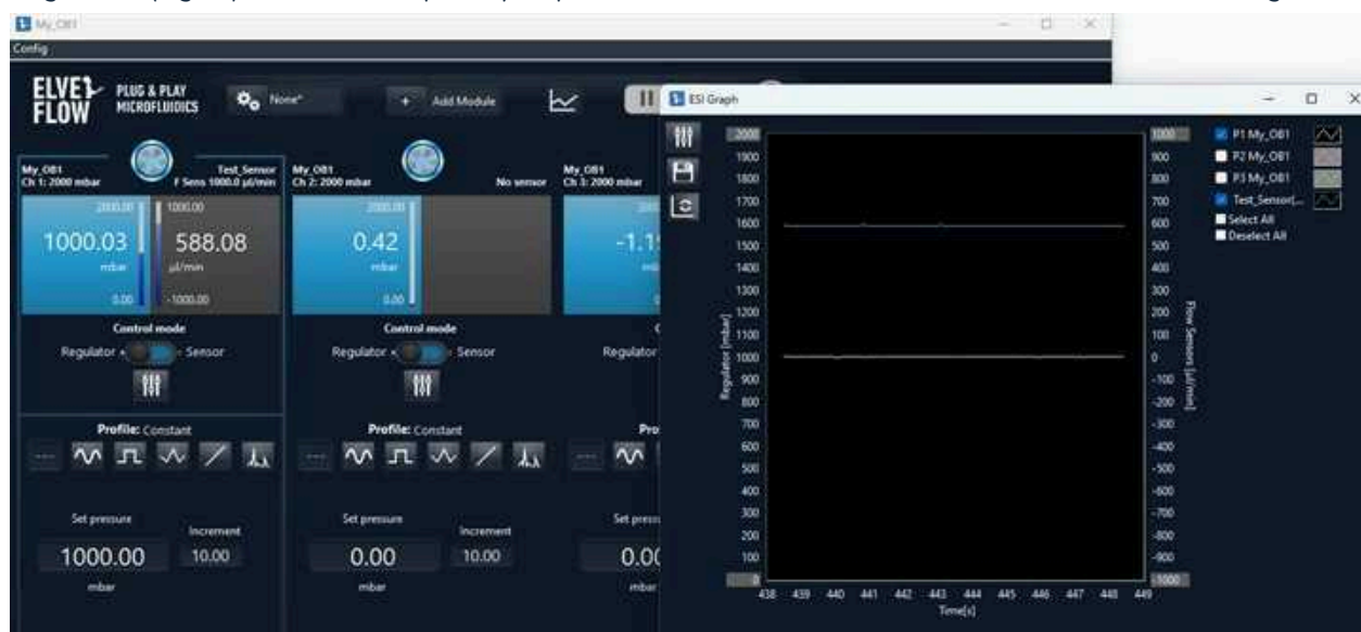
Fig 19. Stability of the flow rate at mid pressure range
