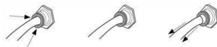
Fig 7. How to disconnect OB1 push-in fittings
