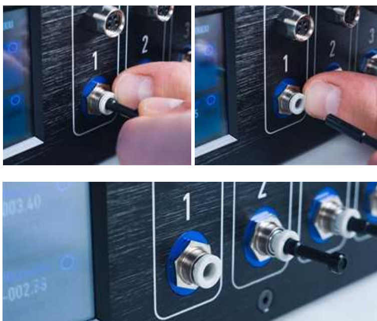
Fig 12. How to disconnect push-in plugs from pressure outlets.
