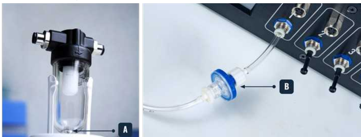
Fig 20. OB1 maintenance: replace the filters at least once a year
