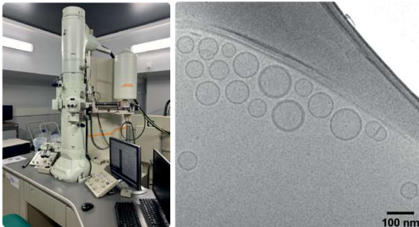
Figure 19: Cryo-TEM setup (left) and example image (right) of the produced LNP using a Herringbone micromixer.
