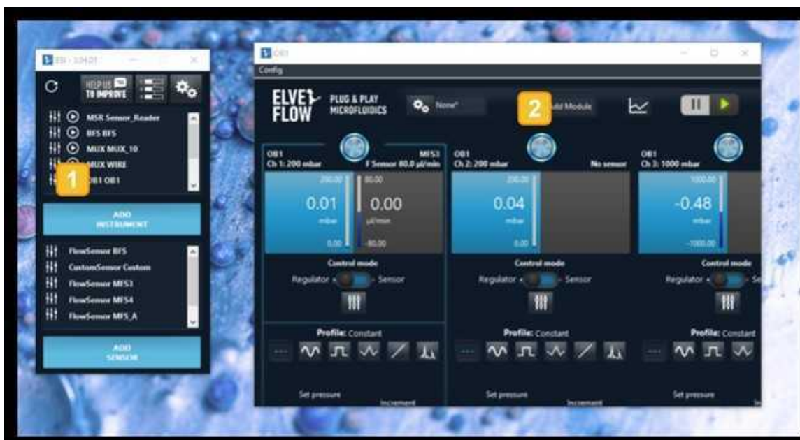
Fig 6. How to reach and open the Sensor Calibration module in ESI.
