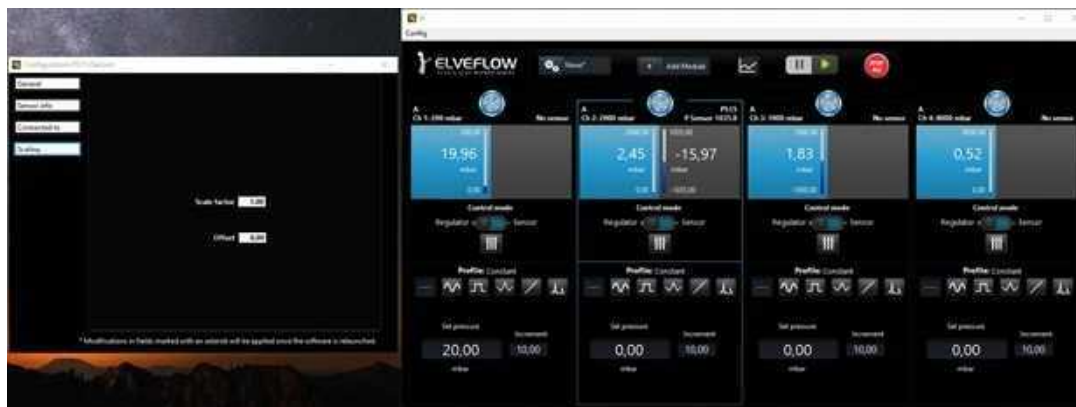
Fig 8a. The MPS Scale Factor and Offset fields can be reached in the "Scaling" tab of the MPS settings.
