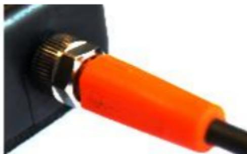
2. Connect the male part of the cable to the female connector on your instrument.
