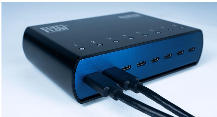
Fig 1. The MUX Wire valve controller can control up to eight microfluidic valves.
