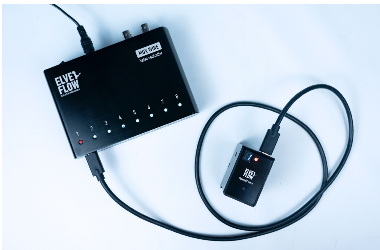
Fig 7. Example of a 2/2 normally closed (NC) valve connected to the first slot of the MUX Wire valve controller and shown on the LED display slot 1 (red). The red light on the MUX Wire and the valve indicate that the valve is in a “closed” position.
