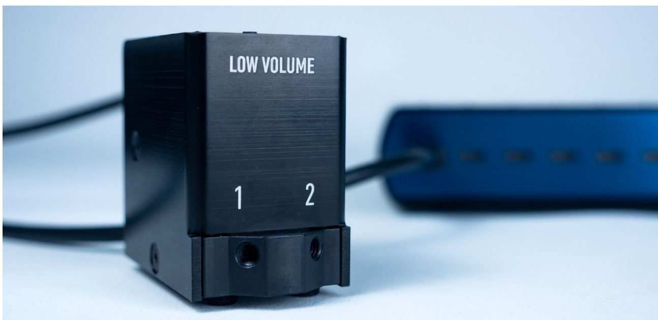
Fig 2. A closeup of a microfluidic valve that can be controlled by the MUX Wire valve controller (in the background).
